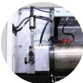
Output pressure transducers activate the discharge module to avoid overpressure on the system
